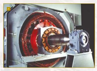
Brushless exciter rotor mounted on shaft of low speed synchronous motor Poles mounted on spider rim Slow speed pedestal bearing machine with brushless exciter rotor and stator Spider rim used to hold poles on slow speed motor
