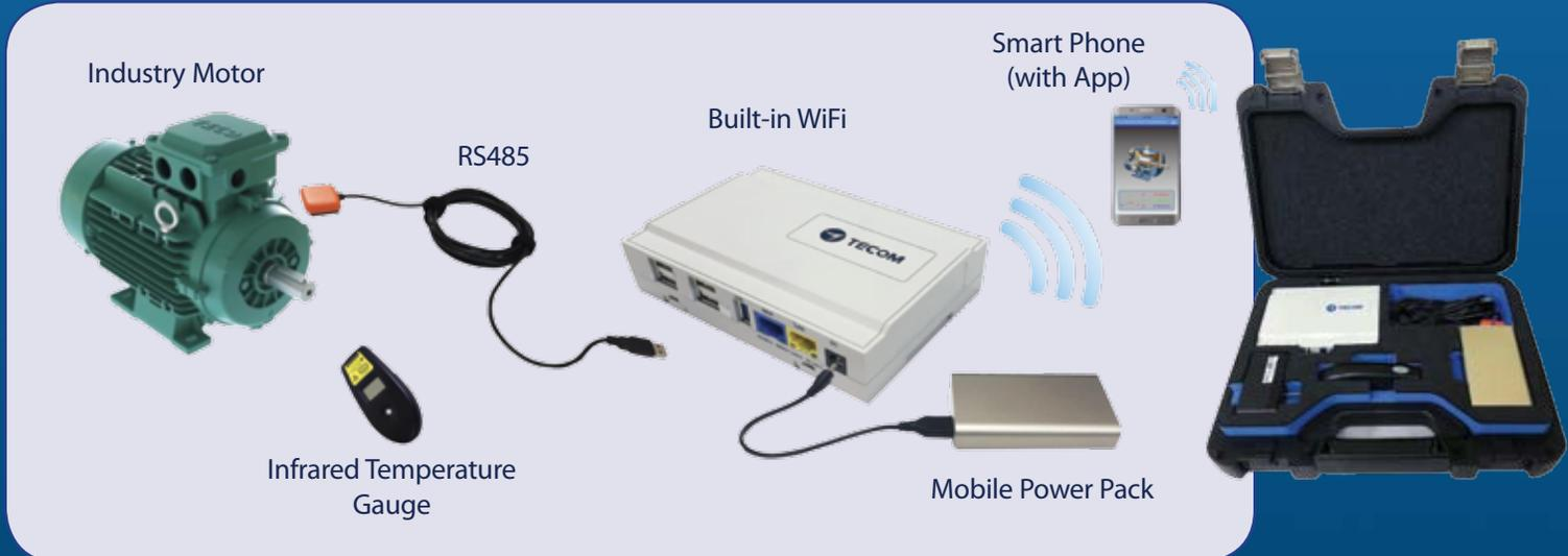
The portable case contains an IoT (Internet of Things) gateway, smart vibration sensors and a rechargeable mobile power pack with a 12 hour battery pack. This allows technicians to carry the device onsite for measurement diagnosis operations.
