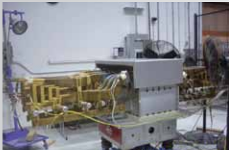
TECO Aging Test of 8 MW Wind Generator Stator
