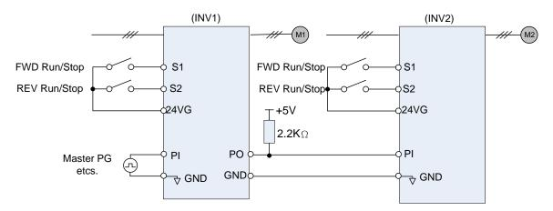
Figure 4.4.32 Speed follower using two inverters
