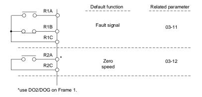
Figure 4.4.25 Multi-function digital output and related parameters
