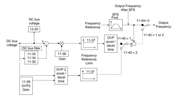
Figure 4.4.91 OVP operation
