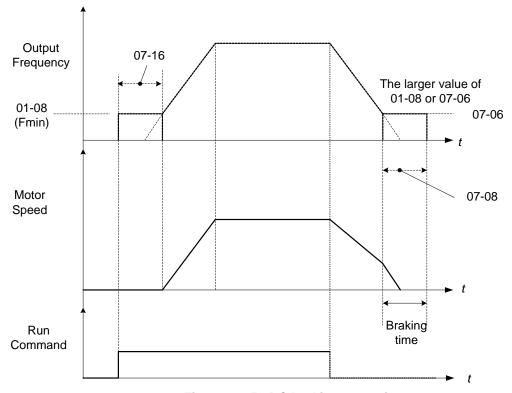
Figure 4.4.57 DC braking operation
