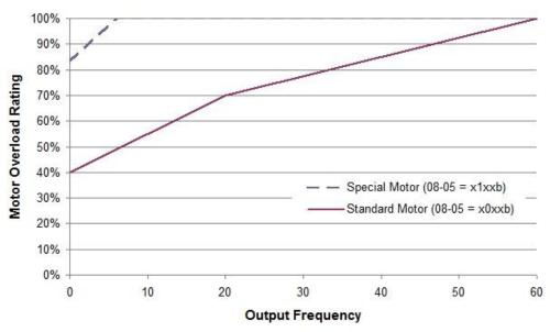
Figure 4.4.72 Motor overload rating at different output frequencies
