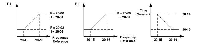
Figure 4.4.112 ASR gain setting (SLV mode)
