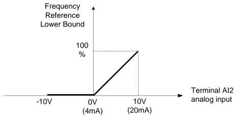
Figure 4.4.47 Adjustment of lower limit of frequency reference
