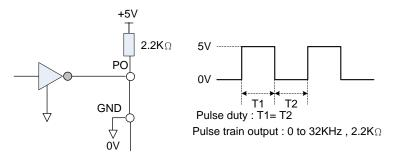
Figure 4.4.30 Pulse output signal level
