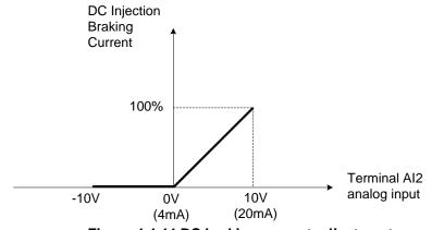
Figure 4.4.44 DC braking current adjustment
