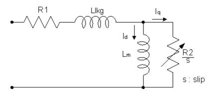
Figure 4.4.15 Y-equivalent model an induction motor
