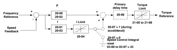
Figure 4.4.109 ASR block diagram (SV mode)
