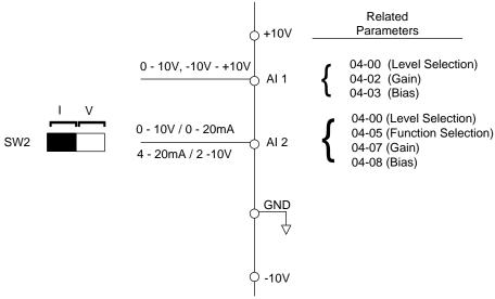
Figure 4.4.35 Analog inputs and related parameters
