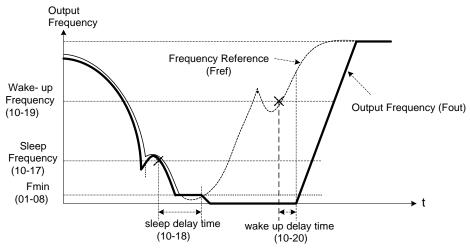
Figure 4.4.83: (b) Timing diagram PID sleep / wakeup
