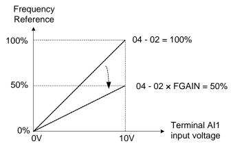
Figure 4.4.39 Frequency reference gain adjustment (example)
