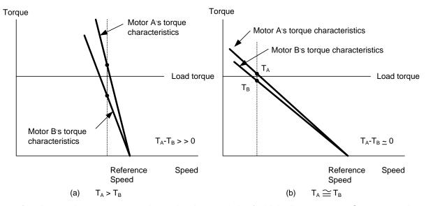
Droop function can be used to approximate the characteristic of a high slippage motor. Set 11-52 to the
