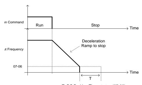
T: DC Braking Time at stop (07-08)
