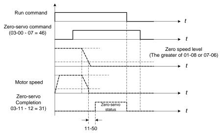
Figure 4.4.96 Zero servo operation
