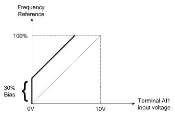
Figure 4.4.41 Frequency Reference bias adjustment (example)
