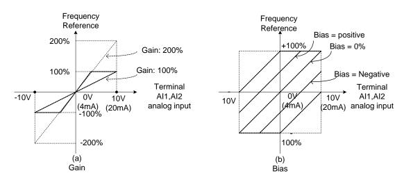
Figure 4.4.36 Gain and bias operations (for frequency reference signal)
