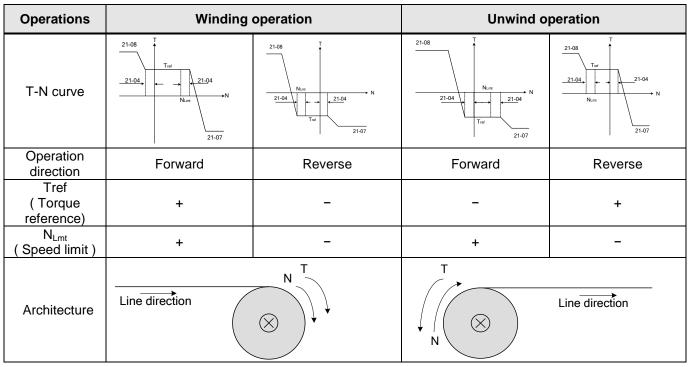
Figure 4.4.126 Winding and roll-out operations
