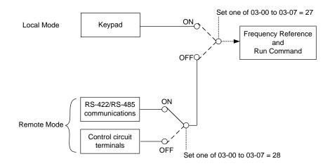
Figure 4.4.23 Remote mode operation selection
