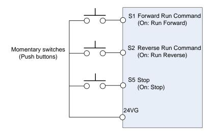
Note: Terminal S1, S2 and S5 must be closed for a minimum of 50ms to activate operation.
