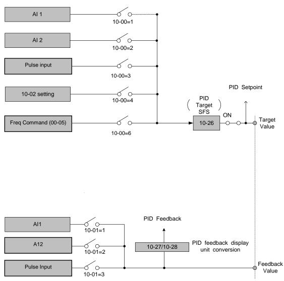
Figure 4.4.80 PID input selection
