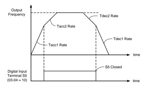
Figure 4.4.7: Terminal S5 switch between Tacc1/Tacc2 and Tdec1/Tdec2
