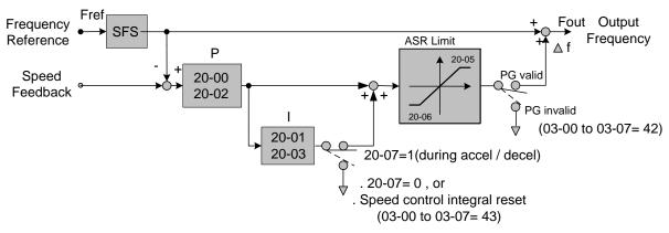
Figure 4.4.107 ASR block diagram (V/F + PG)
