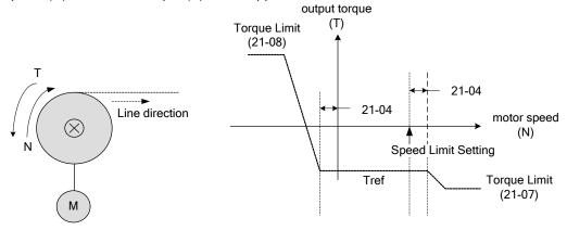
Figure 4.4.125 Unwind operation
