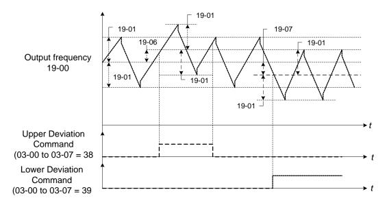
Figure 4.4.106 Upper/Lower offset operation
