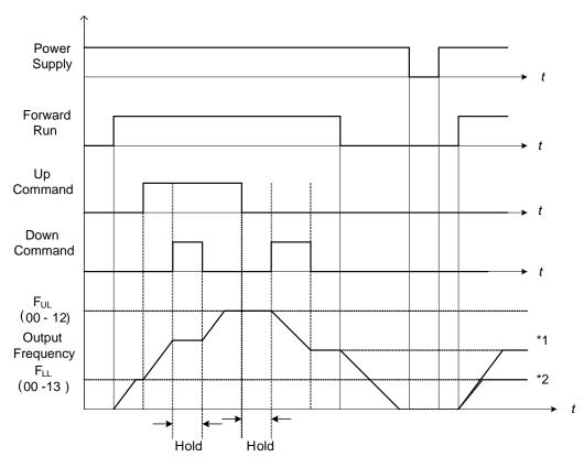
Figure 4.4.20 Up / Down command timing diagram
