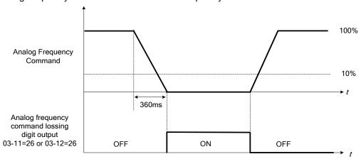
Figure 4.4.93 Operation in reference frequency loss
