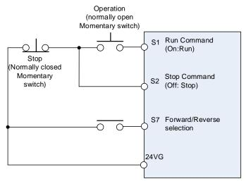
Figure 4.4.2 wiring example of 3-wire
