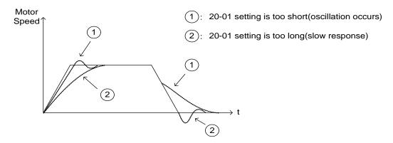
Figure 4.4.114 The response of ASR integral time
