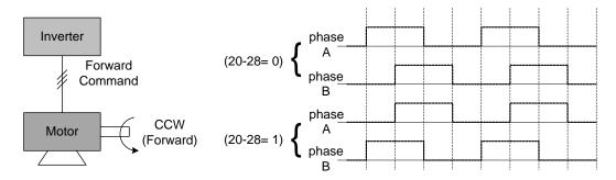
Figure 4.4.118 PG and motor rotation direction
