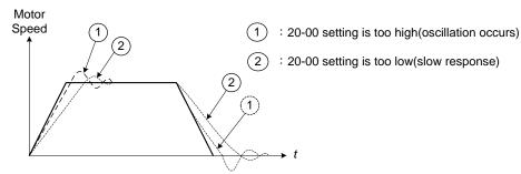
Figure 4.4.113 System response of ASR proportion gain
