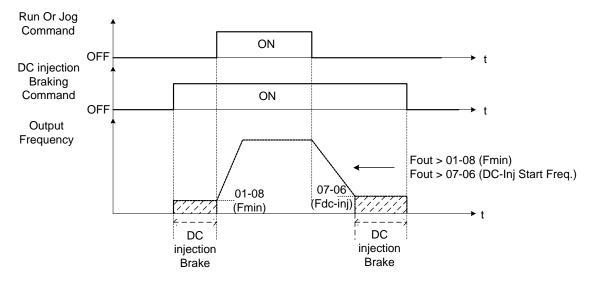
Figure 4.4.24 DC braking timing diagram
