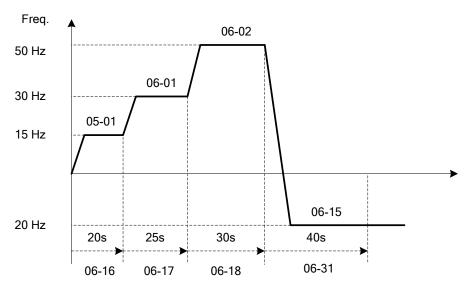
Figure 4.4.54 Single cycle automatic operation (continuous)
