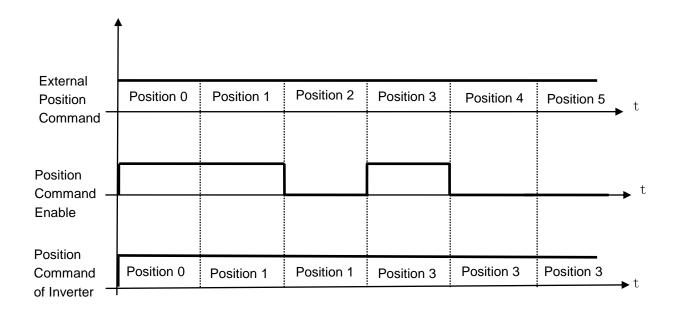
Fig. 4.4.131 Position Enable Diagram
