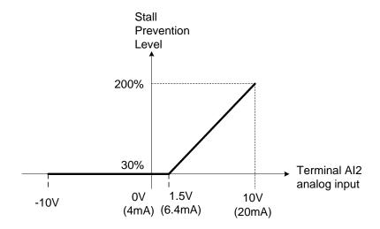
Figure 4.4.46 Stall prevention level adjustment in operation
