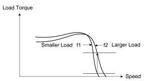
Figure 4.4.99 Slip compensation output frequency
