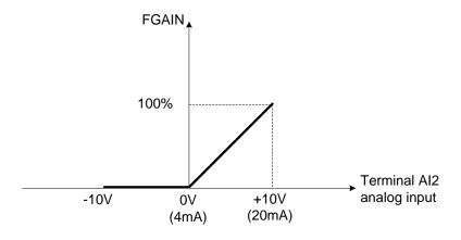
Figure 4.4.38 Frequency gain adjustment
