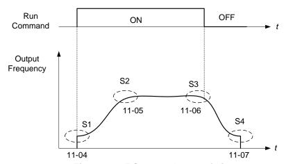
Figure 4.4.85 S curve characteristic
