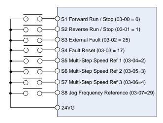
Figure 4.4.17 Control Terminal Wiring Example
