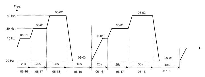
Figure 4.4.53 Periodic automatic operation
