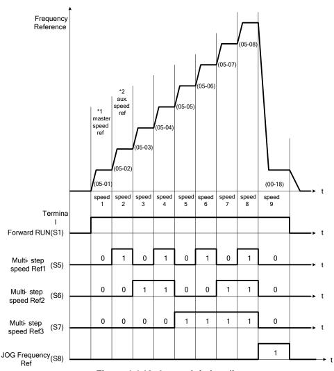
Figure 4.4.18: 9-speed timing diagram
