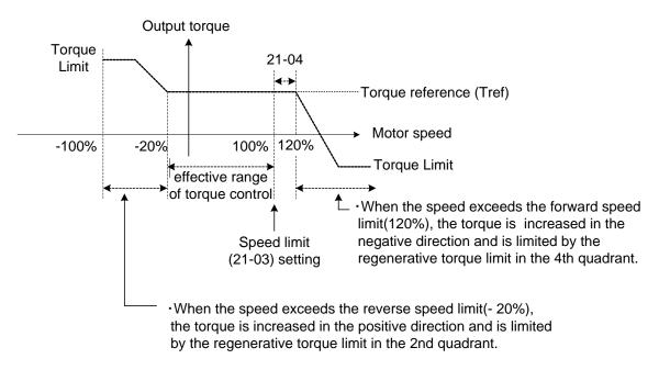
Figure 4.4.123 Speed limit setting (Example 2)
