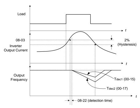
Figure 4.4.70 Stall prevention selection in operation
