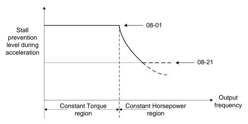
Figure 4.4.68 Stall prevention level and limit in acceleration
