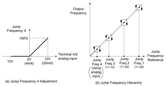
Figure 4.4.48 Jump frequency 4 Setting Operation
