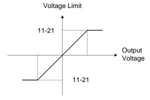
Figure 4.4.89 Voltage limit value of commissioning operation
