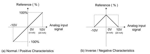
Figure 4.4.10 Positive/negative analog input as main frequency reference command.
