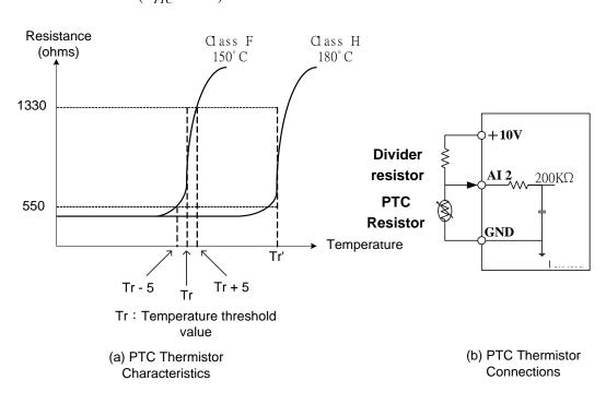
Figure 4.3.65 (a) PTC Thermistor Characteristics (b)PTC Thermistor Connections
