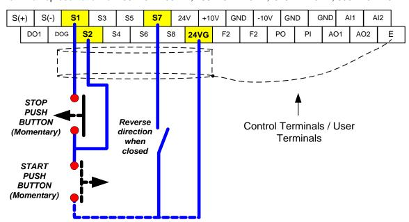
**Note:** Stop mode selection can be set with parameter 07-09, default is **deceleration to stop**.
