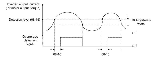
Figure 4.4.73 Over-torque detection operation
