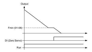
Figure 4.3.129 Zero-servo positioning
