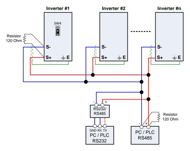
Wiring diagram RS485 Modbus RTU Network
