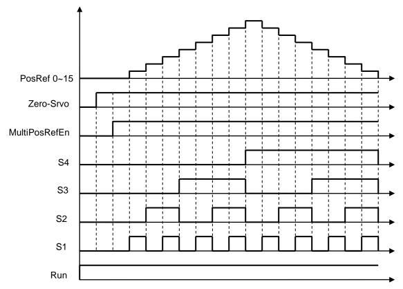
Figure 4.4.130 Multi-positioning logic diagram
