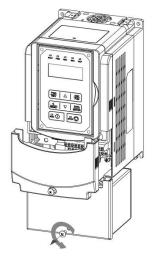
Step 3: Unscrew filter section
