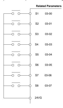
Figure 4.4.16 Multi-function digital input and related parameters
