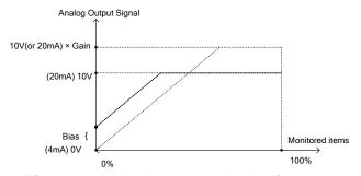
Figure 4.4.51 Analog output level adjustment
