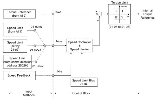
Figure 4.4.121 Block figure of the torque control
