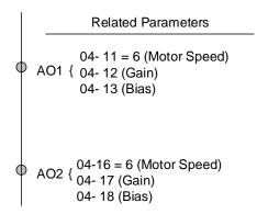
Figure 4.4.111 Analog output setting
