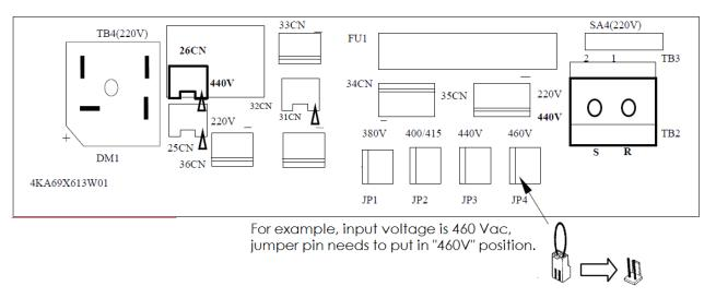
The inverter input voltage range of the A510 600V class models ranges from 575 to 690Vac. In these models the cooling fan is directly powered from the power supply. Inverter models A510s-6175~627 requires the user to select the correct jumper position based on the inverter input voltage ("690V" is the default position for these models). Please select the correct
