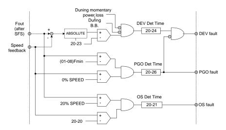
Figure 4.4.117 Logic diagram PG feedback failure detection
