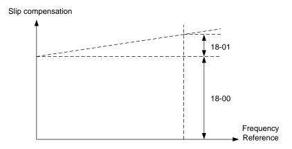
Figure 4.4.102 18-00/18-01 Slip compensation gain versus frequency reference
