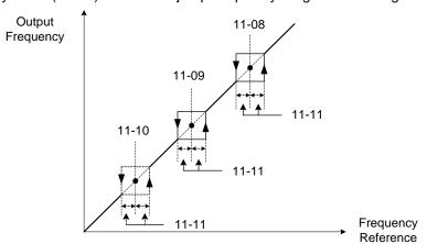
Figure 4.4.86 Jump frequency operation
