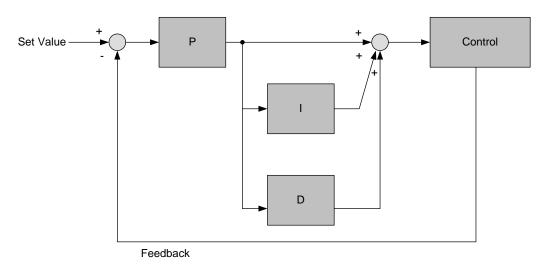
Figure 4.4.79 Basic PID control
