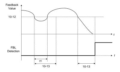
Figure 4.4.82 PID feedback loss detection
