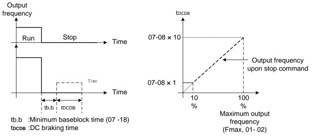
Figure 4.4.60 DC braking to stop
