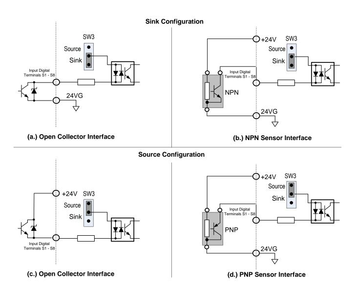
Fig. 3.17.3 Sink / Source Configurations
