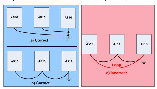
Fig. 3.12.1 Inverter Grounding
