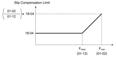
Figure 4.4.100 Slip compensation limit
