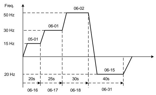
Figure 4.4.52 Single cycle automatic operation (stop)
