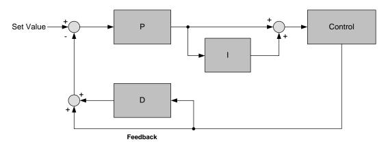
Figure 4.4.78 PID control for feedback differential value
