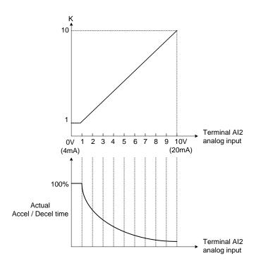
Figure 4.4.43 Acceleration / deceleration time reduction coefficient
