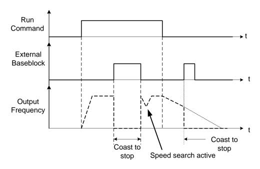
Figure 4.4.22 External base block operation
