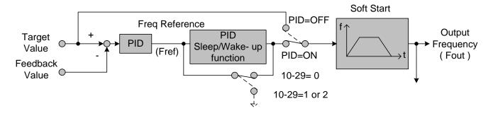
Figure 4.4.83: (a) PID control bock diagram
