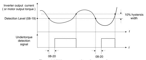
Figure 4.4.74 Low torque detection operation
