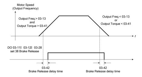
It is recommended to be with starting and stopping frequency locked function (11-43~11-46), shown as the following figure:
