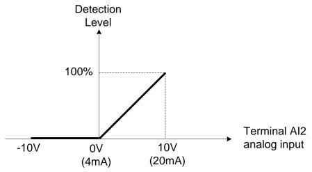
Figure 4.4.45 Over-torque detection level adjustment
