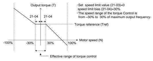
Figure 4.4.122 Speed limit setting
