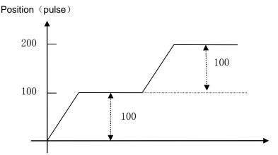
Figure 4.4.132 the absolute type diagram
