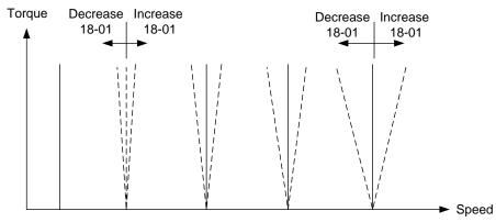
Figure 4.4.103 18-01 Effect on torque speed curve
