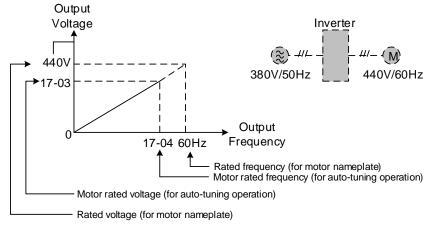
Figure 4.4.98 Rated voltage and frequency settings
