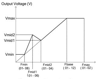
Figure 4.4.13 Torque boosting
