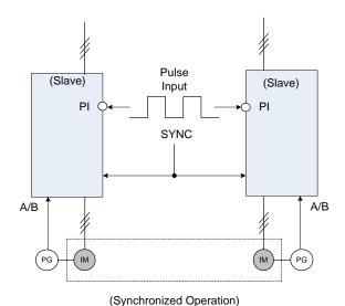
Figure 4.4.33: Synchronized operation of using pulse input
