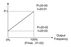
Figure 4.4.110 ASR gain setting (V/F+PG)
