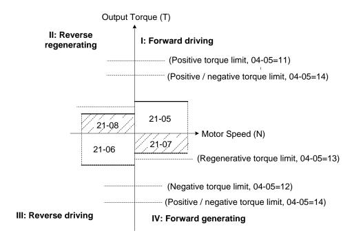
Figure 4.4.128 Analog input torque limit (Al2)
