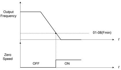
Figure 4.4.26 Zero-speed operation
