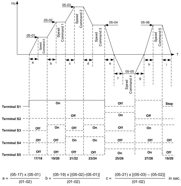
$$a = \frac{(05-17) \times (05-01)}{(01-02)} \quad b = \frac{(05-19) \times [(05-02)-(05-01)]}{(01-02)} \quad c = \frac{(05-21) \times [(05-03)-(05-02)]}{(01-02)} \quad \text{in sec.}$$
