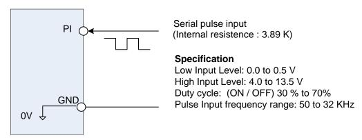
Figure 4.4.5 Frequency reference from pulse input
