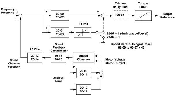
Figure 4.4.108 ASR block diagram (SLV mode)
