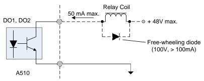
Fig. 3.17.2 Photo-Coupler Connected to an External Relay
