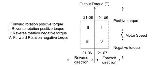
Figure 4.4.127 Torque limit setting
