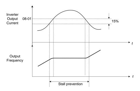
Figure 4.4.67 Stall prevention during acceleration
