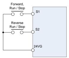
Figure 4.4.1 wiring example of 2-wire
