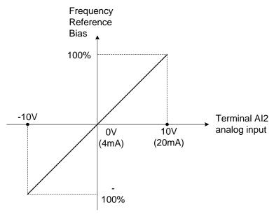
Figure 4.4.49 Operation of being added to Al1 as bias
