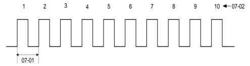
Figure 4.4.55 Automatic restart interval
