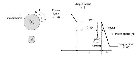
Figure 4.4.124 Winding operation
