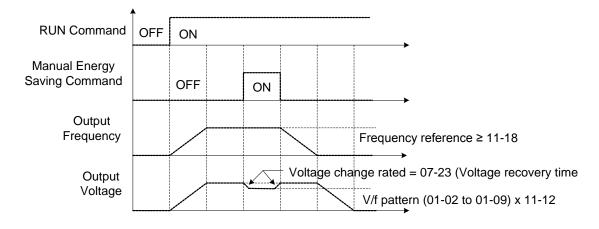
Figure 4.4.88 Manual energy saving operation
