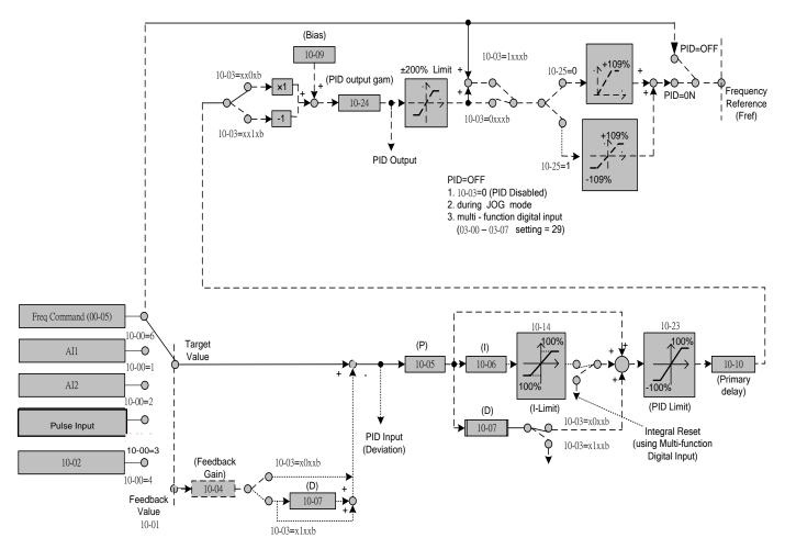
Figure 4.4.81 PID control block diagram
