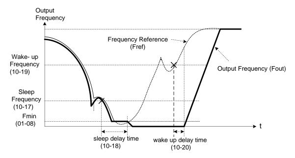
Fig. 4.4.83 PID Sleep Function
