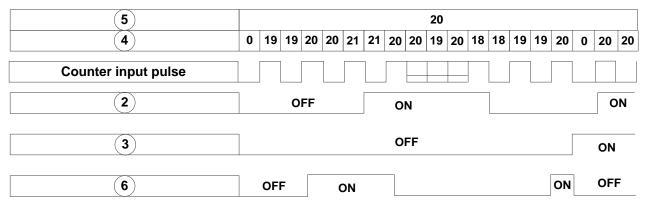
**Note:** In this mode the internal counter may increase past the counter compare value, unlike mode 1 where the internal counter value is limited to the counter compare value.
