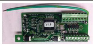
The A510 product has a standard RS485 port with RTU Modbus protocol. Optional protocol communication cards are available.
