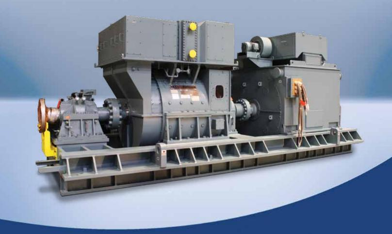
The *Ocean Researcher V*, a state-of-the-art 2700T research vessel, was built by Jong Shyn Shipyard in Taiwan for the Taiwan Ocean Research Institute. The first of its kind, this vessel has a unique propulsion system which includes tandem TECO-Westinghouse DC/AC motors powered by Siemens Blue Drives. The hybrid DC/AC propulsion set operates on DC power in Super Quiet mode and with a combination of DC & AC power for normal operation, making it ideal for advanced Ocean Research Vessels.
