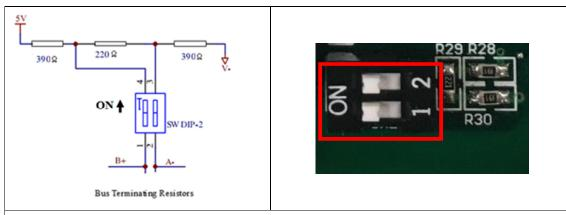
The first and last station of the PROFIBUS bus must be connected to the bus, and the bus terminal resistor must be turned on.
