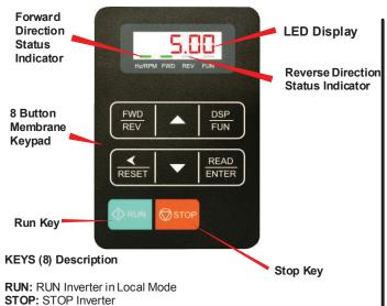
FWD/REV: Switch between Forward and Reverse operation
