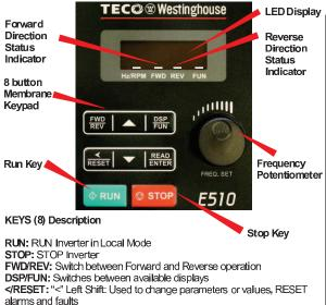
**READ/ENTER:** Used to display the preset value of parameters and to save changes
